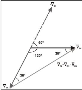
$$V_L = |\vec{V}_{RS}| = 2 \times |\vec{V}_{RN}| \times \cos 30^\circ$$
